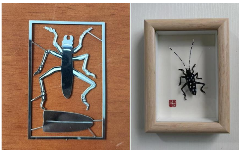
Figure 6 Semi-finished products etched by an etching machine and finished Chinese iron painting finished by hand processing. Note: Photographed by researcher
