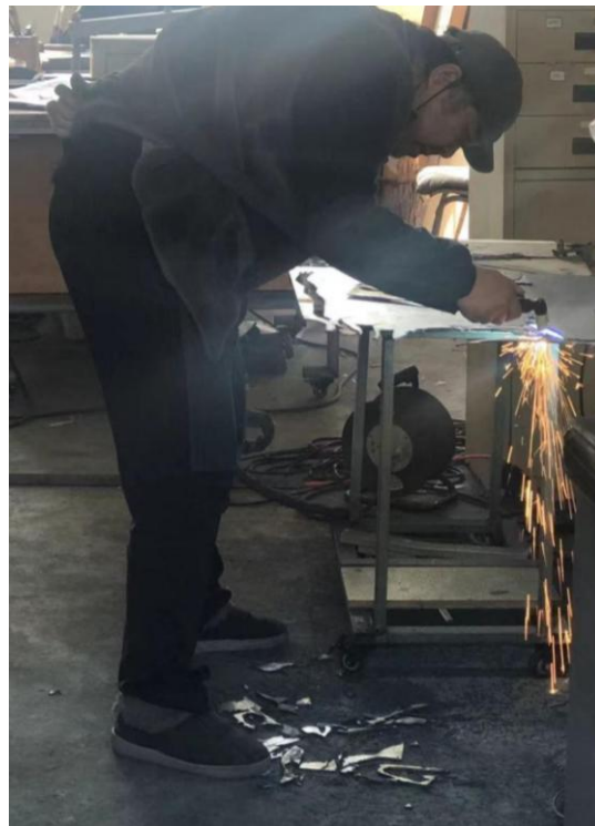
Figure 4 Chinese iron painting inheritors use plasma equipment to cut iron Note: Photographed by researcher
