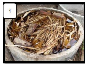
1 Soak the hemp bark in water for approximately 3 hours
