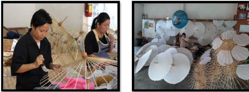
Figure 5 Shows the umbrella cladding process. (A) Apply Tako rubber to the umbrella frame. (B) White paper cladding on the umbrella frame.
