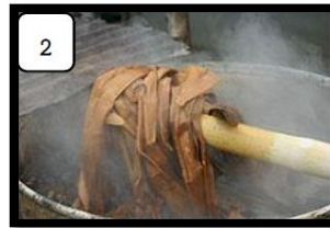
2 Bring to a boil in a solution of sodium hydroxide. (NaOH) about 3 hours and rinse with water until the solution is not base
