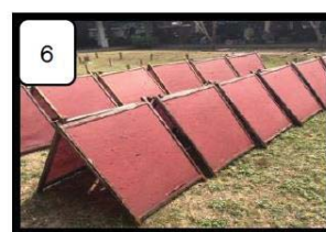
6 to dry approx. 2 hours, then peel off the mulberry paper from the mold to get a sheet of paper out.
