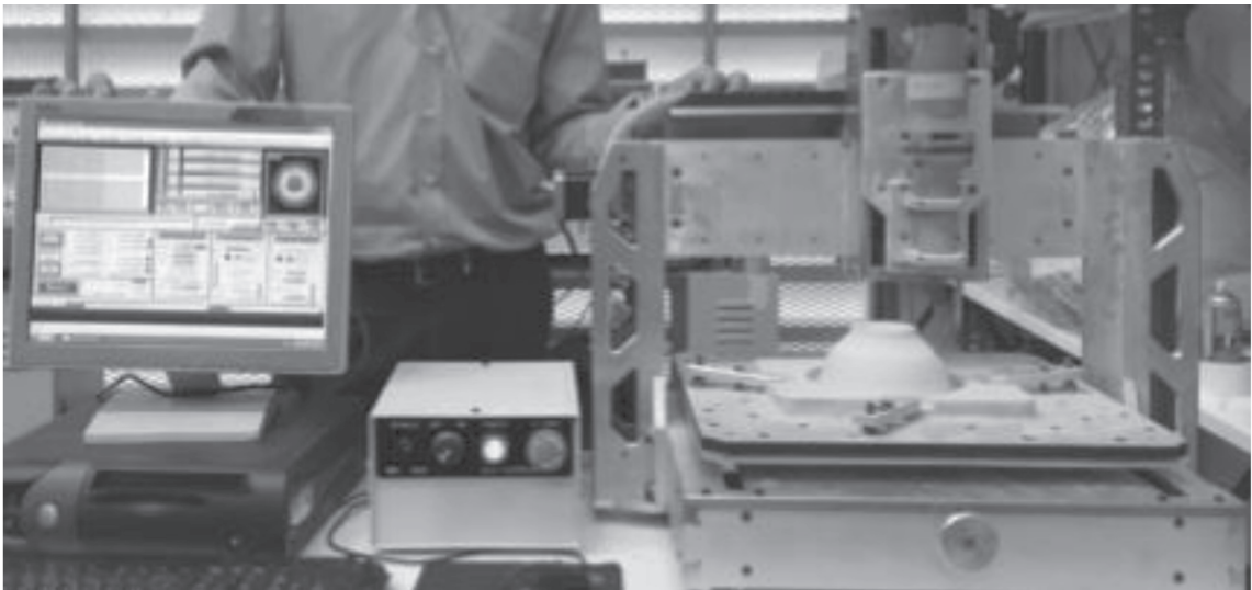
Figure 10 Example of a 3-axis CNC machine for molding ceramic cups/ bowls
