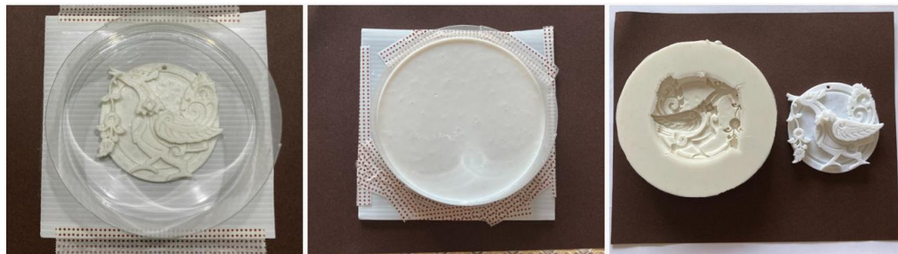
Figure 9 Making a silicone rubber mold
