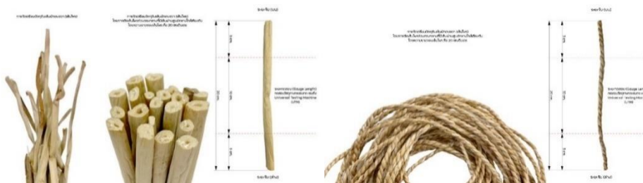
Figure 2 Preparing raw materials of water hyacinth in 2 forms: 1) Round strands, and 2) Spiral strands
