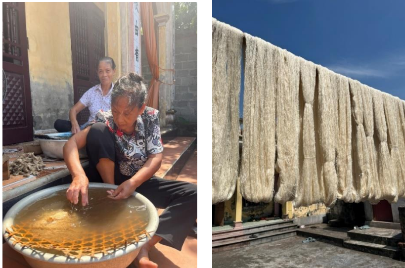
Figure 2a Artisans making the threads from the cover of the cocoons at Nam Cao Village and Figure 2b Silk threads made by artisans at Nam Cao Village (Photos by Authors)
